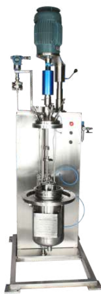
10L with pneumatic vessel raising lowering
