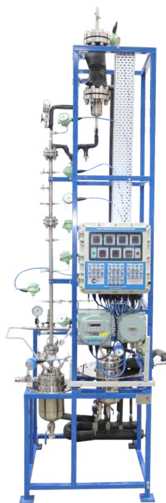
5L high pressure ex-proof distillation skid
