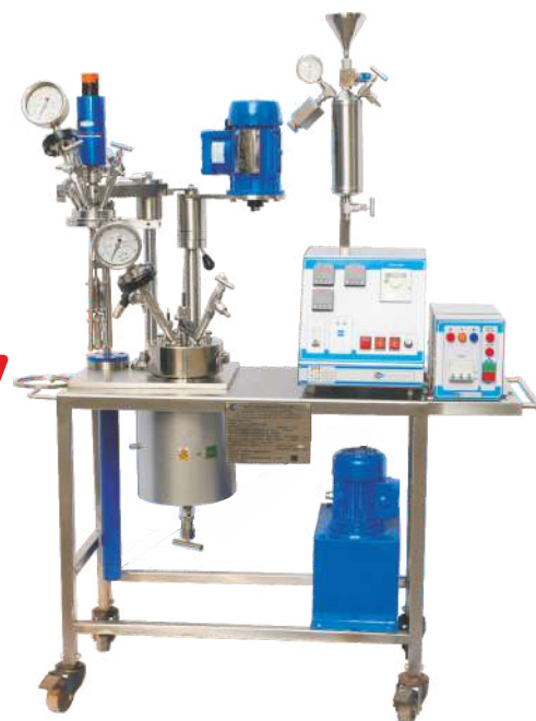
2L autoclave with separate head for weight loss method & electrochemical corrosion studies
