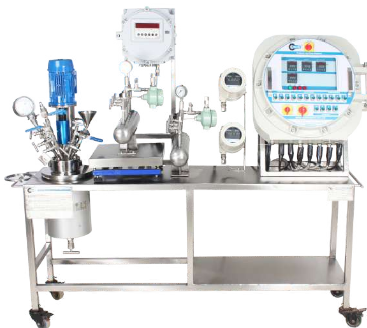
EO-PO pilot plant with ex-proof fittings
