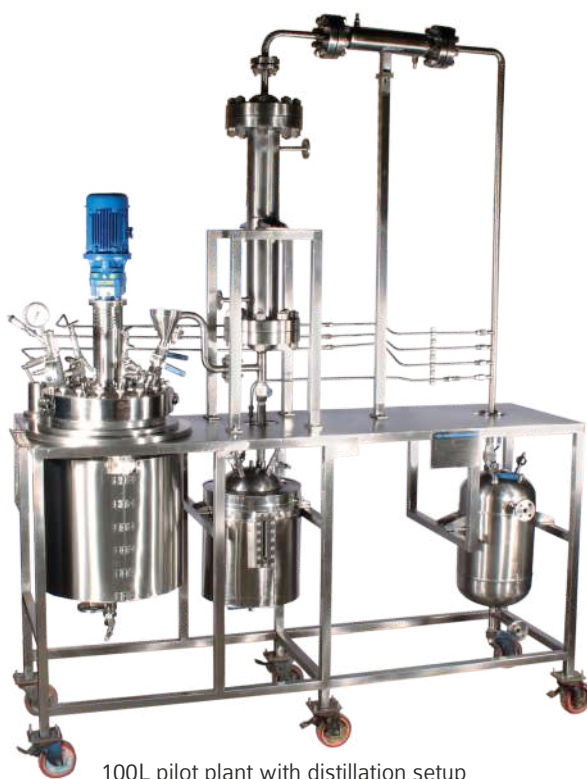
100L pilot plant with distillation setup
